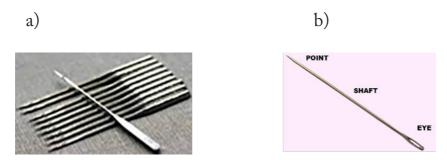
Figure 5.7: Various types of needles: (a) Sewing machine needles, (b) hand sewing needle
