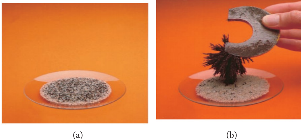
Figure 2.16 (a) the mixture contains iron fillings and sand. (b) A magnet separates the iron fillings from the mixtures.
