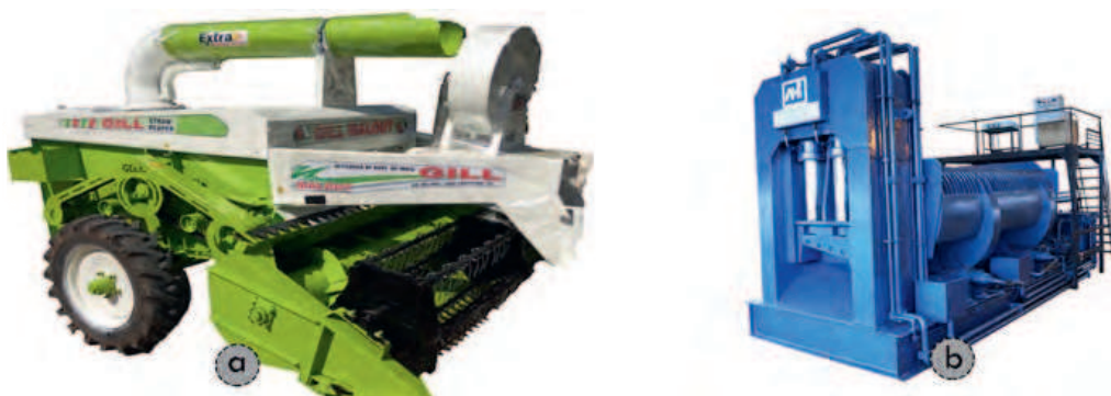
Figure 14.4. a) straw collector, b) baler
